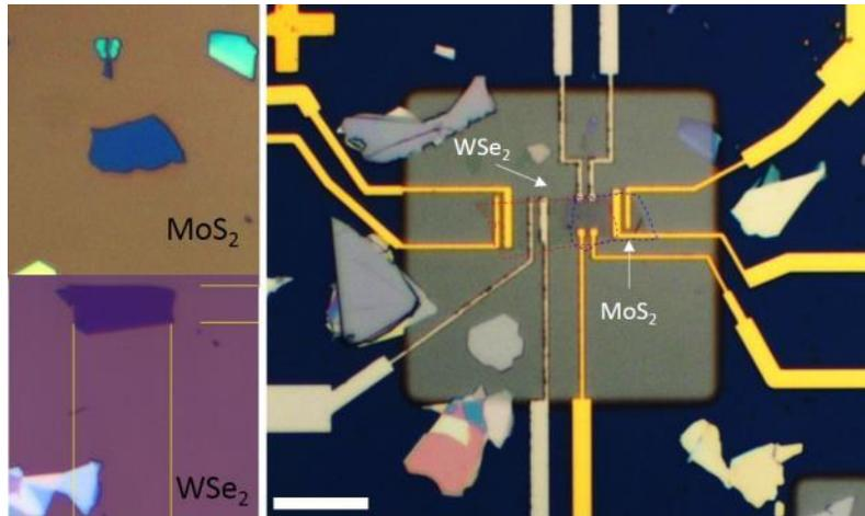
**Figure S4:** Optical images of representative exfoliated MoS<sub>2</sub> and WSe<sub>2</sub> flakes as well as the final MoS<sub>2</sub>/WSe<sub>2</sub> hetero-FET fabricated in a 90 nm deep SiO<sub>2</sub> via coated with 10 nm HfO<sub>2</sub>. Flakes are contacted with Au and Pd. The scale bar is 10 μm.
