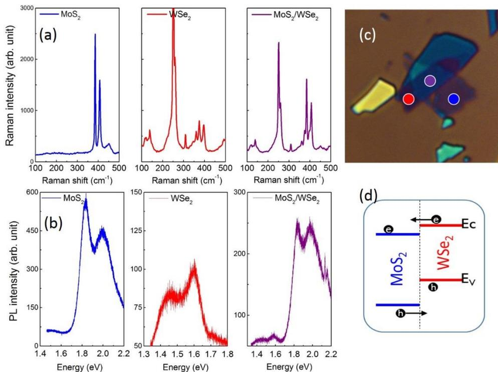
**Figure S2:** (a) Raman spectrum of the sample taken at the different points marked in (c). (b) Photoluminescence spectrum of the sample at the same points marked in (c). (c) Optical image of the
