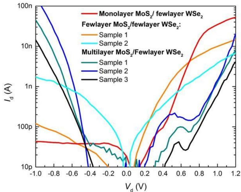
**Figure S8:**  $I_d-V_d$  of several MoS<sub>2</sub>/WSe<sub>2</sub> hetero-FETs with different MoS<sub>2</sub> and WSe<sub>2</sub> thicknesses fabricated in this work.
