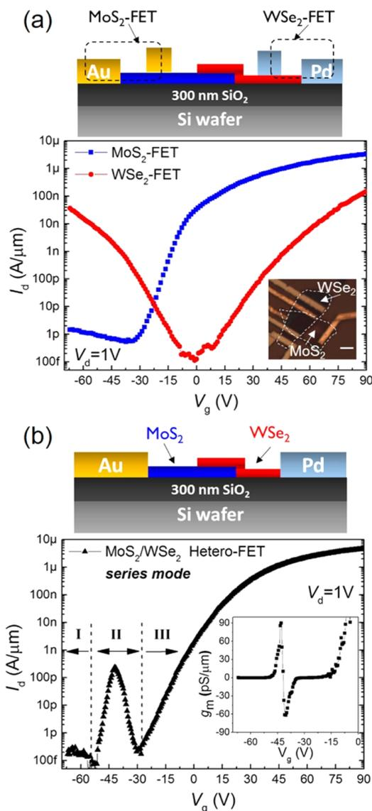
**Figure 1.** (a) Transfer characteristics ( $I_d-V_g$ ) of a back-gated few-layer MoS<sub>2</sub>- and WSe<sub>2</sub>-FET. The inset shows an optical image of a typically stacked MoS<sub>2</sub>/WSe<sub>2</sub> FET. The scale bar is 5  $\mu\text{m}$ . (b)  $I_d-V_g$  of the MoS<sub>2</sub>/WSe<sub>2</sub> heterojunction FET in the series measurement mode. The inset shows the transconductance centered around the peak in region II. The schematics show the corresponding device measurement setups.
