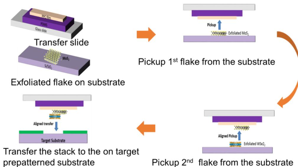
**Figure S1:** Schematic of the heterostructure fabrication by the dry transfer method.
