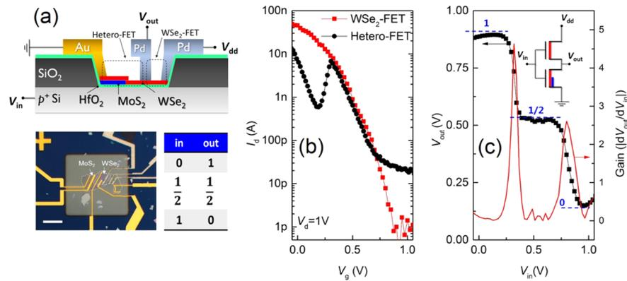
**Figure 4.** (a) Schematic of the ternary inverter, an optical image of the device, and an input–output table of the inverter. (b) Comparison of  $I_d$ – $V_g$  curves of the hetero-FET and WSe<sub>2</sub>-FET shown in (a). (c)  $V_{out}$  versus  $V_{in}$  plot of the ternary inverter showing three distinct levels of logic. The inset shows a circuit schematic of the inverter.
