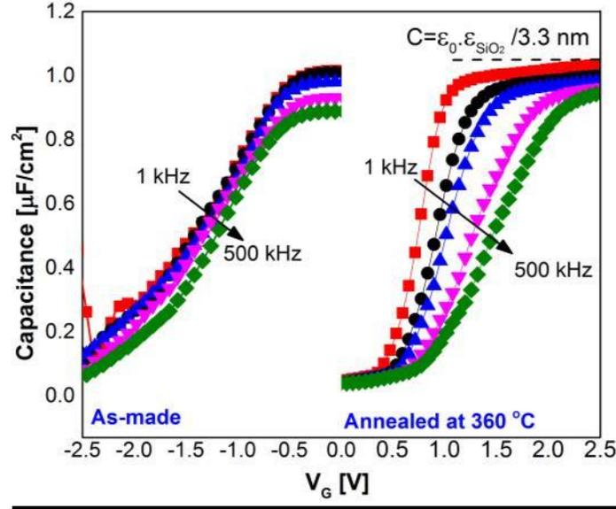
**Figure S5:** *As-made and after-annealing capacitance–voltage characteristics of a multilayer MoS<sub>2</sub> capacitor at different frequencies in the 1 to 500 kHz range.*
