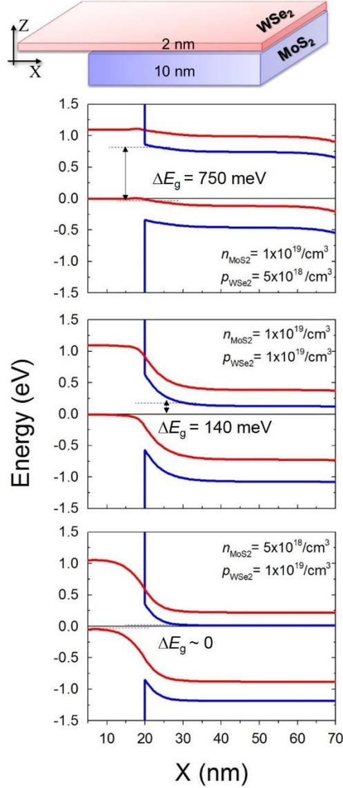
**Figure S7:** Schematic of a 2 nm WSe<sub>2</sub>/10 nm MoS<sub>2</sub> heterojunction and its calculated in-plane band diagrams with three different MoS<sub>2</sub> and WSe<sub>2</sub> charge concentration combinations.
