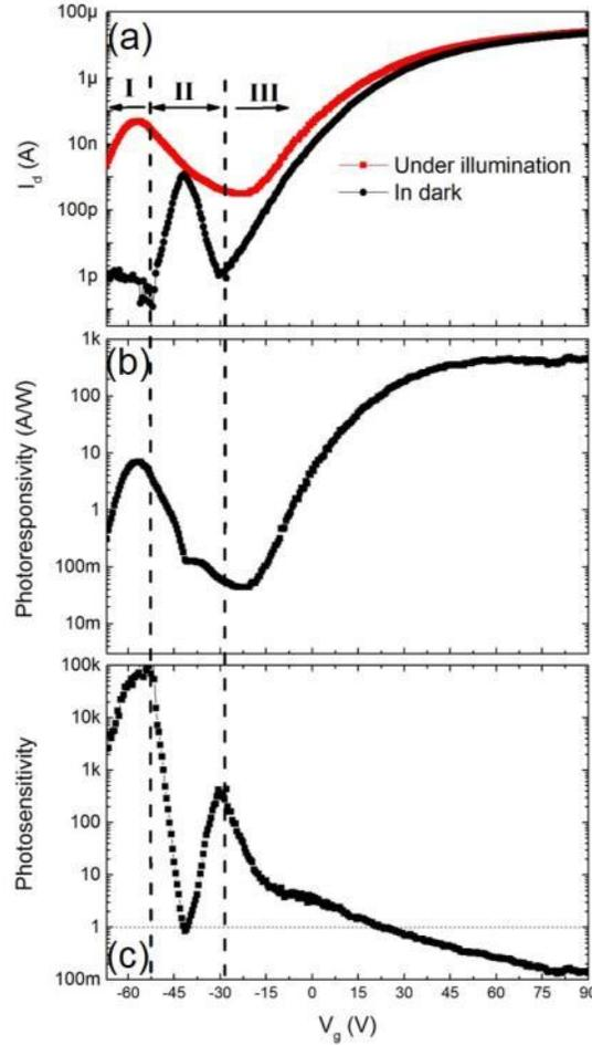
**Figure S3:** (a) Transfer characteristics of the in-series MoS<sub>2</sub>/WSe<sub>2</sub> hetero-FET (also shown in Figure 1(b)) in the dark and under illumination. (b) Photoresponsivity and (c) photosensitivity under a white light power intensity of 0.03 W/cm<sup>2</sup>.
