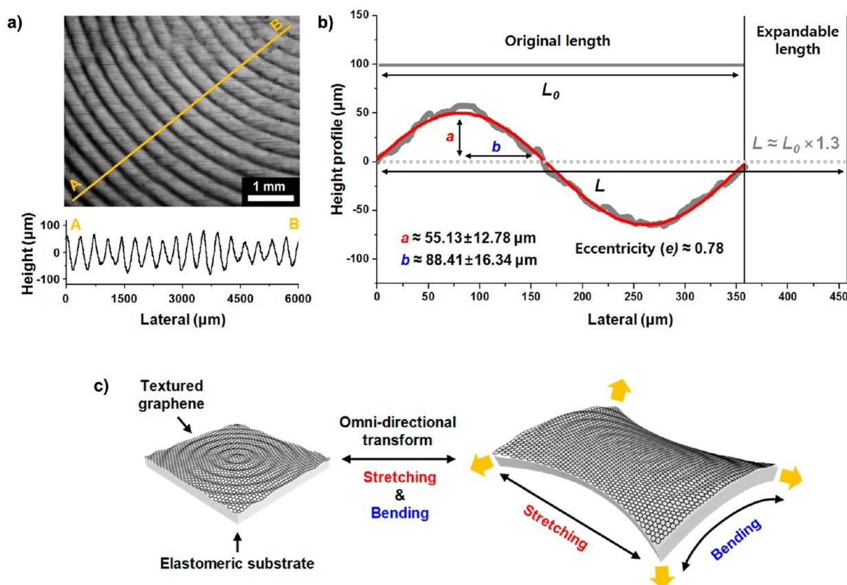
**Figure 4.** (a) OM image of a graphene/PDMS film with a concentric circle pattern and two-dimensional line scan profile taken vertically through the yellow line on the OM image. (b) Enlarged surface topography of a graphene/PDMS film. Fitting curve is indicated by the red line. (c) Schematic illustration of the transformation of the graphene/PDMS film under applied forces.
