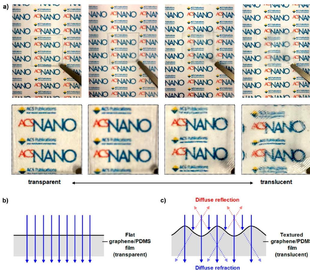
Figure 2. (a) Optical hazing on the textured graphene/PDMS film. Photographs were taken at different distances between the image and the textured graphene/PDMS film. The distances are 0, 0.5, 1.0, and 3.0 cm, respectively. Differences occur between transparency and translucency. The schematic illustration on the (b) left has high transparency, whereas the image on the (c) right has diffuse reflection and high transparency (translucency).
