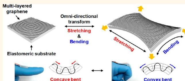
Stretchable and transparent electrodes have been touted as a key component of the “next generation of electronics”.<sup>1–3</sup> These electrodes can be formed into nonplanar forms to make them suitable for applications in flexible and wearable electronics such as rolled-up displays, smart clothing, skin-like sensors, stretchable solar cells, and other easily collapsible gadgets.
