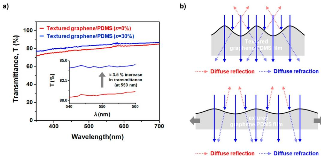
Figure 3. (a) Optical transmittance spectra of textured graphene samples under different tensile strains. (b) Schematic illustration of the transmittance mechanism for textured graphene at 0% and 30% tensile strain.
