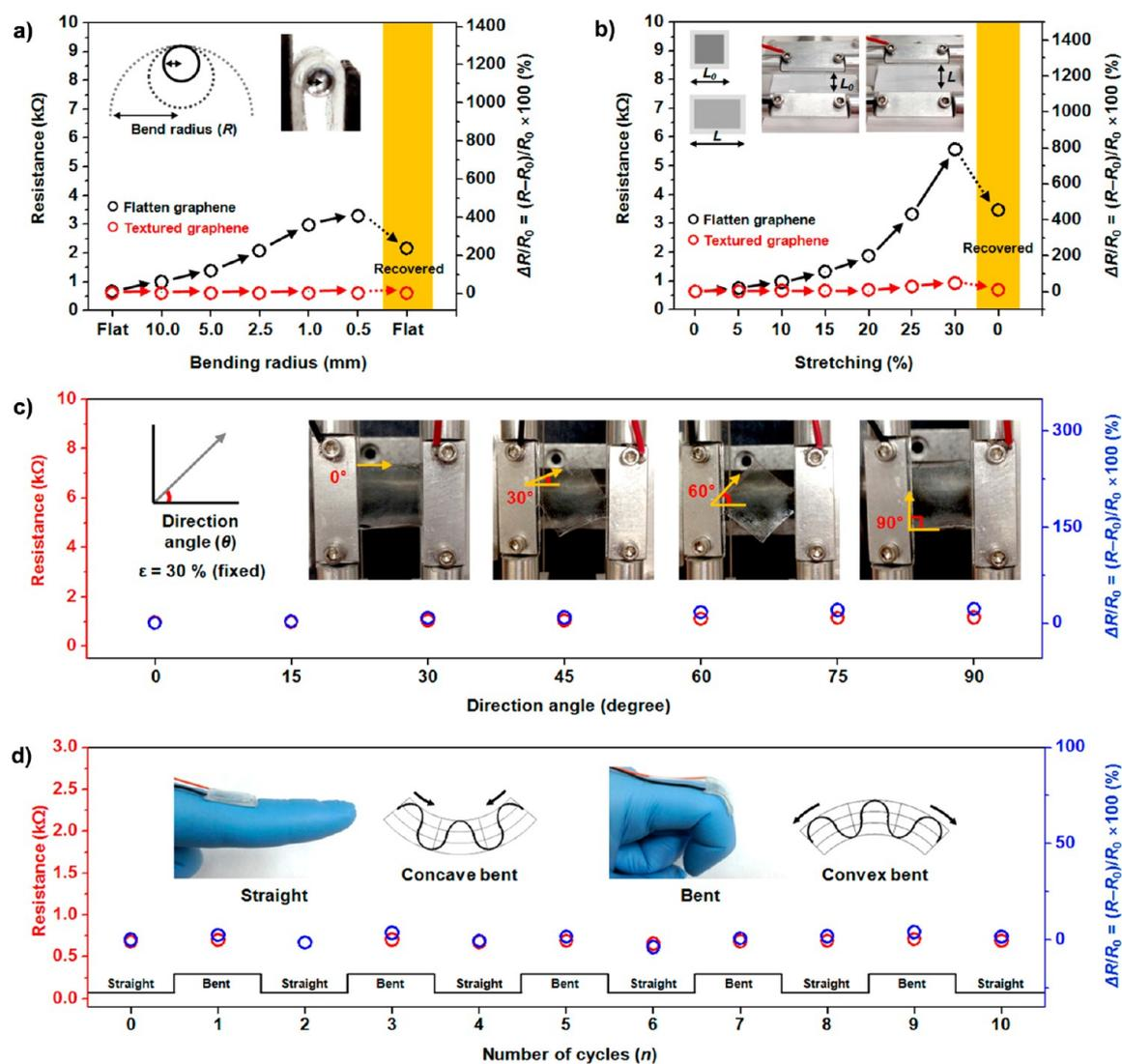
**Figure 7.** Variation in resistance of a textured graphene/PDMS film as a function of (a) bending radius and (b) tensile strains (insets: actual test images for a graphene/PDMS film). (c) Variation in resistance of a textured graphene/PDMS film under various stretching angles (from 0° to 90°). Stretching tests were performed under a fixed tensile strain of 30%. (d) Variation in resistance of a textured graphene/PDMS film as a function of a finger-bending cycle.
