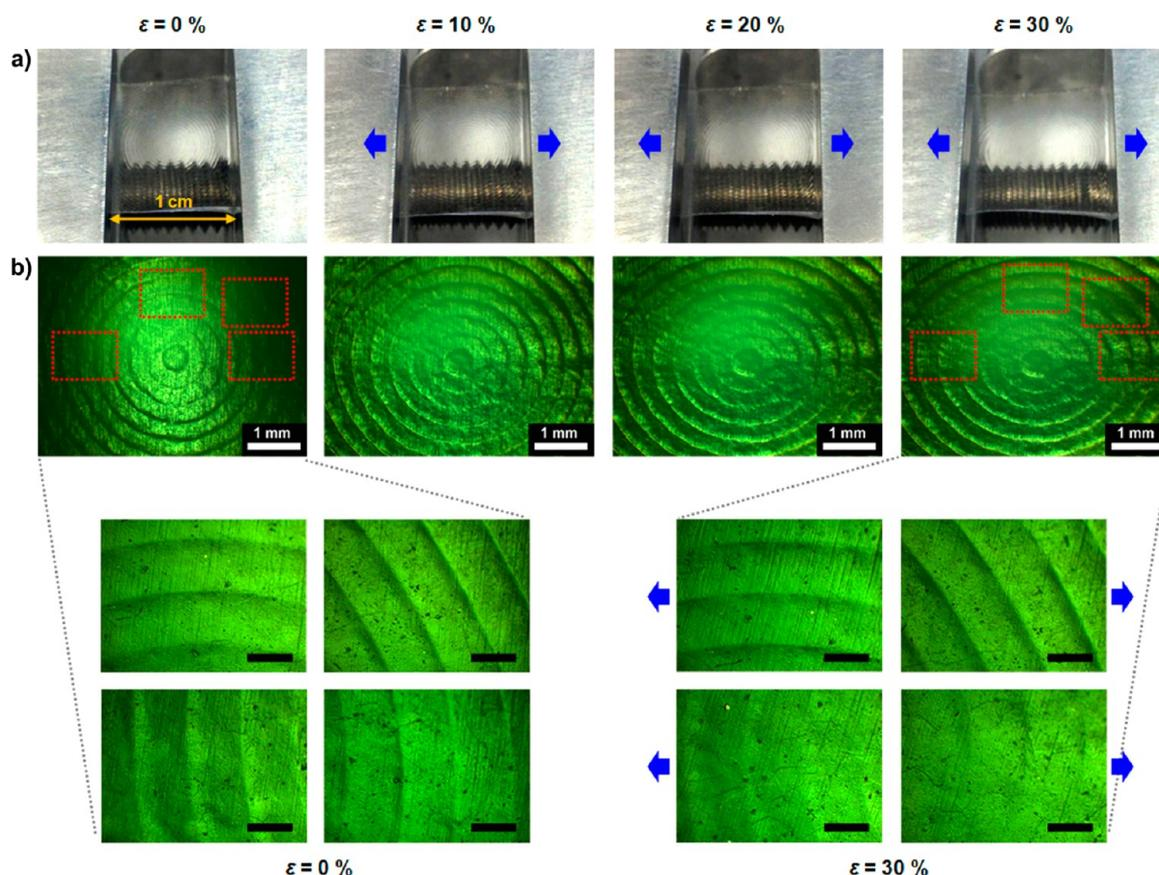
**Figure 5.** (a) Stretching test images for the textured graphene/PDMS film. Stretching tests were performed under various tensile strains (from 0% to 30%). (b) Corresponding OM images for the textured graphene/PDMS film under various tensile strains. Enlarged optical images were taken at different parts shown in the red boxes (scale bar indicates 200  $\mu\text{m}$ ).
